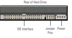
b. With 3.5" drives, attach the free end of the IDE ribbon cable to the back
