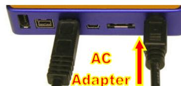
Your Forensic UltraDock is now ready to use! Turn on the unit by moving the power switch to the "I" position. The red drive access indicator will light briefly after the unit is powered up, indicating that the FireWire bridge has successfully established communication with the drive. Thereafter, it will light whenever the drive is accessed.
