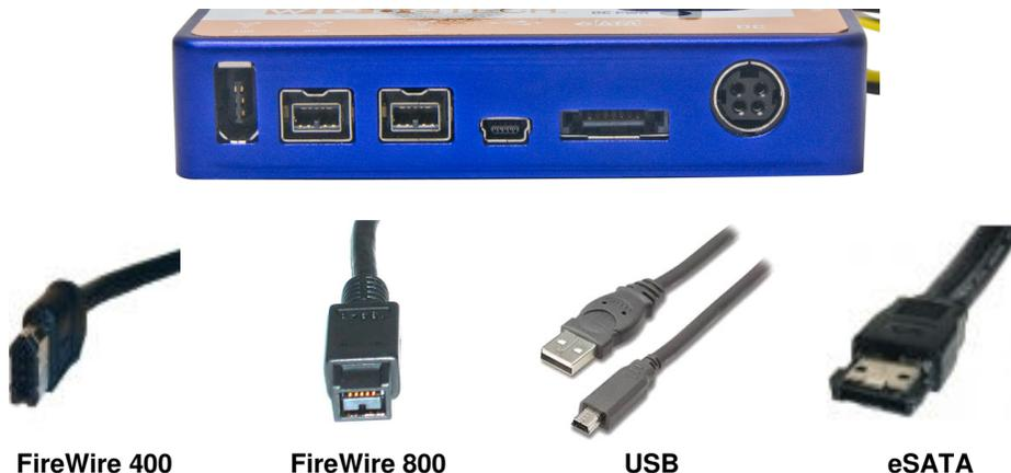
Connect power to the Forensic UltraDock. Use either the included AC adapter or, optionally, you can connect a 4-wire power cable from inside a computer case. This is useful if you wish to access a drive inside a computer without removing it first.
